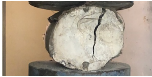
Figure 12. Failure pattern of the basalt textile-confined concrete under tensile test. Source: Authors' own work.
