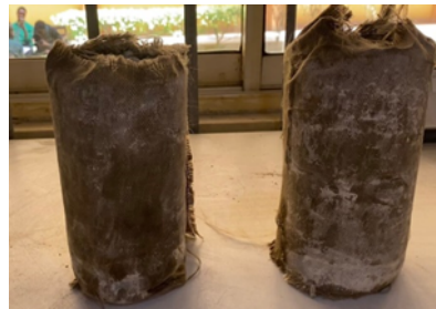
Figure 4. Periwinkle shell lightweight concrete cylinder confined in basalt textile. Source: Authors' own work.
