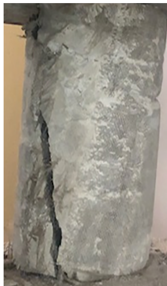
Figure 9. Failure pattern of the basalt textile not confined concrete cylinder under compressive test. Source: Authors' own work.
