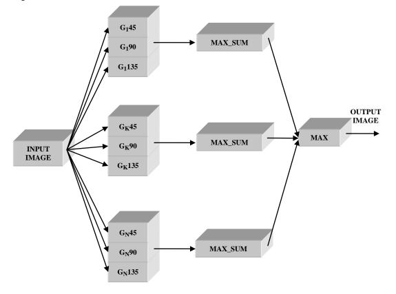
Fig. 2. The block diagram of the gradient computing procedure.
